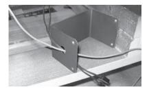
9) Install the plastic bushing over the outside of the hole.
